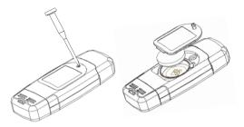
This product uses a CR2450 button battery.Please install the battery before operating the data logger. When battery capacity is not sufficient or during replacing battery, the data logger will stop recording but the recorded data will not be lost. User needs to download the data to PC and replace with a new battery to restart the data logger.
