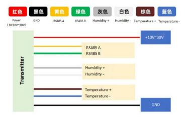
Please check the transmitter wiring to prevent damage to the transmitter due to incorrect wiring! Please wire transmitters with different analog output types according to the diagram below.
